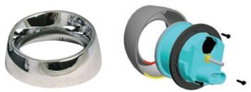
The visor Rim attaches by slipping the rim from the front of the gauge and slipping the bracket from behind, secure the bracket to the rim with screws and your done.
